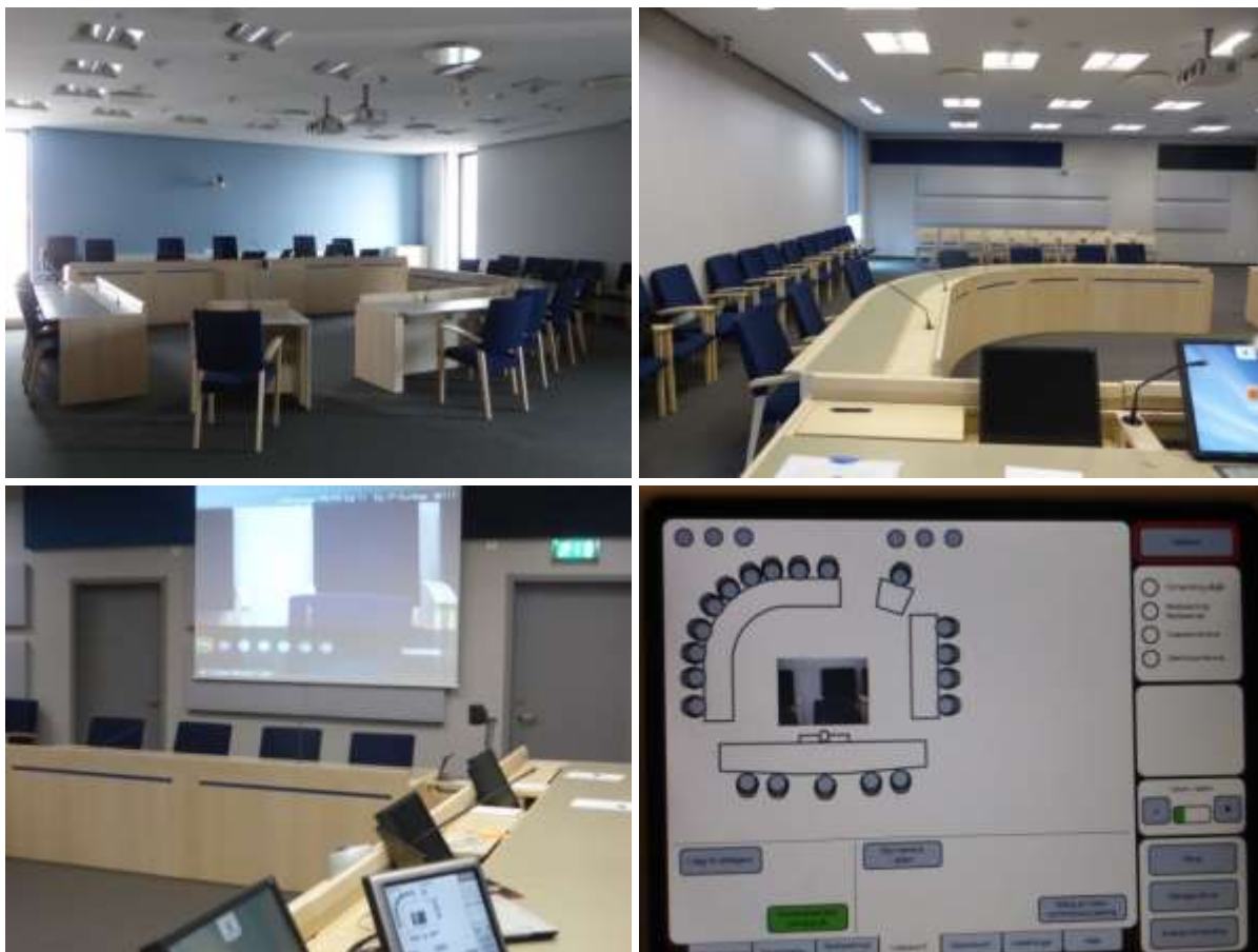
Figure 2 a) Top left: Court view to bench; camera 1 above the bench; b) Top right: Court view from bench; camera 2 at the rear wall; c) Bottom right: projection screen showing remote site (no PiP); c) Bottom left: control touch panel (image from remote site displayed in the middle; camera pre-set positions in the court room)
