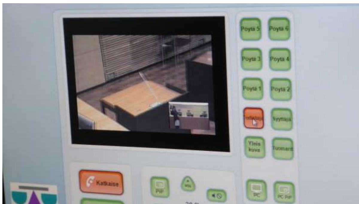
Figure 3: Control panel with preset buttons showing an image of the courtroom with a PIP.
